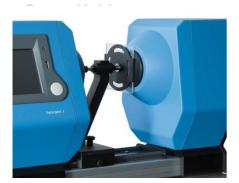
The measurement of haze is used to determine abrasion resistance of transparent materials. The haze-gard **i** Abrasion Holder facilitates positioning of the abraded area in the measurement beam.
